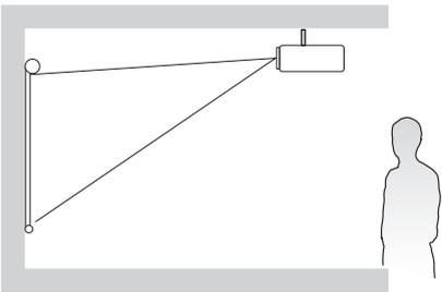
A schematic diagram of a room showing a screen on the wall. A projector is mounted upside down on the ceiling in front of the screen. A person is standing to the right of the screen, looking at it. Lines from the projector indicate the projection area onto the screen. |
