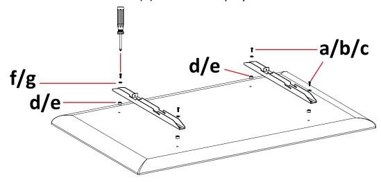
10. Secure the Mini PC bracket onto the stand as shown below.
