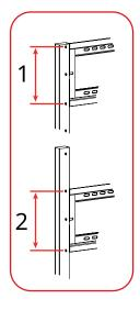
**4.** After choosing the appropriate combination, screw one **M8x16 mm Screw** (**G**) halfway into the middle mounting hole of the chosen combination into each **Column** (**A** & **B**).
