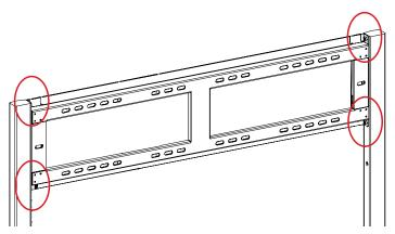
7. Screw one M6x12 mm Screw (H) halfway into each Column (A & B) as shown below.
