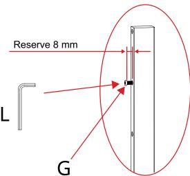
**5.** Hang the **Wall Plate** (**D**) onto the two halfway screwed **M8x16 mm Screws** (**G**). Once hung, fully tighten both **M8x16 mm Screws** (**G**).
