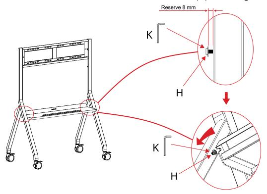
8. Place the Plate (C) onto the two exposed M6x12 mm Screws (H). Fully tighten the two M6x12 mm Screws (H). Using the remaining two M6x12 mm Screws (H), further secure the Plate (C) to the Left (A) and Right Columns (B).
