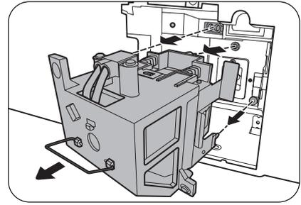
6. Ensure the handle is fully laid flat and locked in place.
