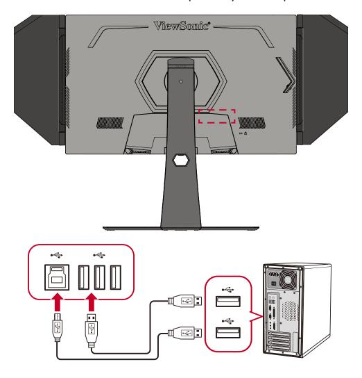
**NOTE:** The USB Type A port next to the USB Type B port can support 5V 2.1A fast charging. The other two USB Type A ports can support 5V 0.9A charging.
