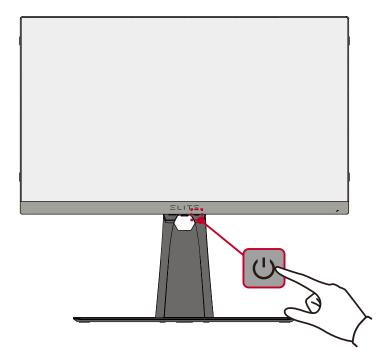
**NOTE:** The monitor will still consume some power as long as the power cord is connected to the power outlet. If the monitor is not being used for a long period of time, please disconnect the power plug from the power outlet.
