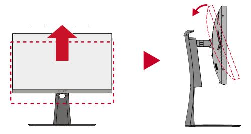
**NOTE:** Ensure the Elite Hood is removed or folded in prior to pivoting.
