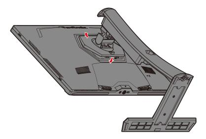
**NOTE:** Ensure the stand is secure and the quick release tab positively clicks into place.
