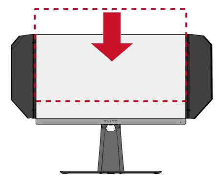
**NOTE:** When adjusting, press down firmly along the adjustment track holding the monitor with both hands on the side.
