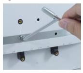
Simply screw the supplied table stand onto the stand screw hole.
