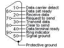
The diagram shows a hexagonal pinout for an RS-232 connector. Pin 1 is at the top, followed by 2, 3, 4, 5, 6, 7, 8, and 9 at the bottom. A legend to the right lists the functions for each pin:
