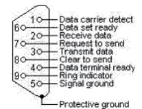
The diagram shows a hexagonal outline representing the RS-232 connector. Inside, numbered pins are connected to specific functions:
