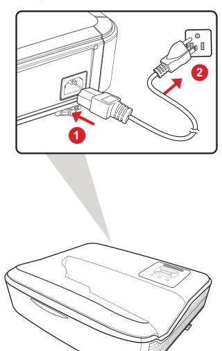
**NOTE:** When installing the projector, incorporate a readily accessible disconnect device in the fixed wiring, or connect the power plug to an easily accessible outlet near the unit. If a fault should occur during operation of the projector, use the disconnect device to switch off the power supply, or disconnect the power plug.
