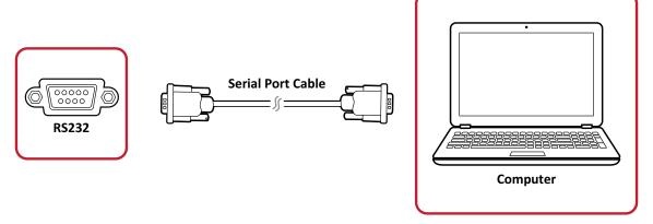
When you use a RS-232 serial port cable to connect your display to an external computer certain functions can be controlled remotely by the PC, including Power On/Off, Volume adjustment, Input select, Brightness, and more.
