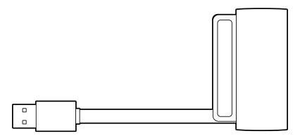
The charger is magnetically attached to the lower right side of the ViewBoard. Connect the charger to the USB 3.0 port on the side of the panel.
