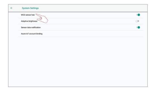
**3.** When WCD and Sensor data notification are turned on, the environmental data will be displayed on-screen.
