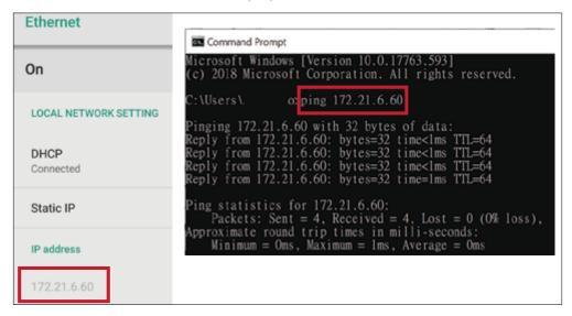
**3.** Log in to the ViewBoard with the client equipment. Input the ViewBoard's IP address.
