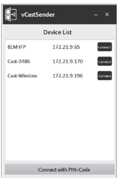
**NOTE:** If the device is not listed, click **Connect with PIN-Code** and input the pin-code displayed on the ViewBoard.
