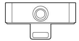
The camera is magnetically attached to the top middle of the ViewBoard. Connect the camera to the USB 3.0 port on the side of the panel as shown below.
