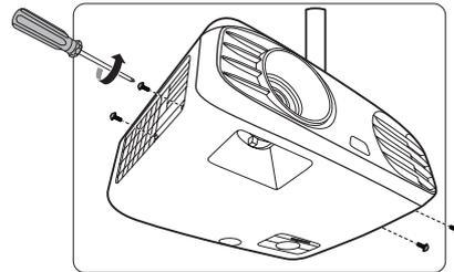
3. Remove the lamp cover and mylar from the projector.
