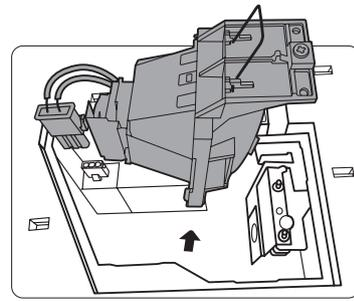
8. As show in the figure, insert the new lamp. Align the lamp using the alignment holes and gently push the lamp into the locked position
