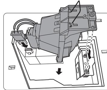
9. Insert the lamp connector and tighten the screw that secures the lamp.
