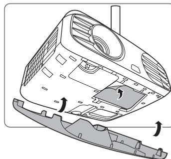
11. Tighten the screws that secure the lamp cover.
