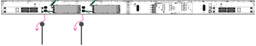
System Control Box Power Cables
