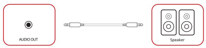
**NOTE:** The display is equipped with two **Audio Out** ports, one can be accessed externally, while the other is accessed by removing the System Control Box Cover.
