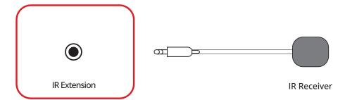
**NOTE:** The **IR Extension** port is accessed by removing the System Control Box Cover.
