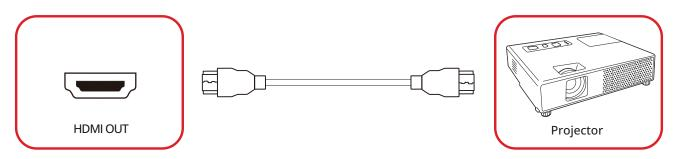
To output video via an external display device, connect an HDMI cable to the **HDMI IN** port of your external display device, and the other end to the **HDMI OUT** port of the display.
