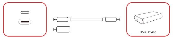
Plug the USB device or storage drive into the USB Type C (
