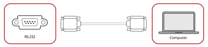
When you use a RS-232 serial cable to connect the display to an external computer or control system, certain functions can be controlled remotely such as: power on and off, volume adjustment, input select, brightness, and more.
