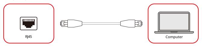
When you use an Ethernet cable to connect the display to an external computer or control system, certain functions can be controlled remotely such as: power on and off, volume adjustment, input select, brightness, and more.
