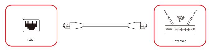
To connect to a network, connect an Ethernet cable to your network, then connect the other end to the **LAN** port of the display.
