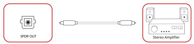
**NOTE:** The **SPDIF Out** port is accessed by removing the System Control Box Cover.
