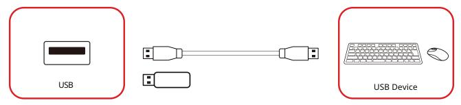
Plug the USB device or storage drive into a USB Type A (**USB 3.0** or **USB 2.0**) port on the display's control panel.
