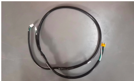
Power Cable of Cabinets "A" and "B"
