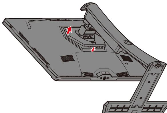
4. Pull down slightly to disengage the hooks and remove the stand.
