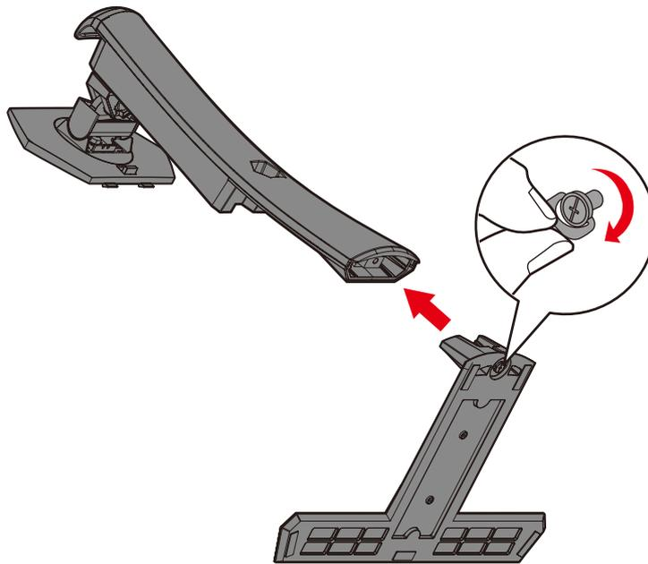
4. Align and slide the upper hooks of the monitor stand into the stand mounting slots as shown in the illustration below:
