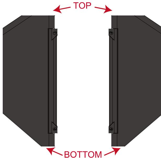
3. Line up each screw of the Elite Hood piece with the screw holes on the side of the monitor.
