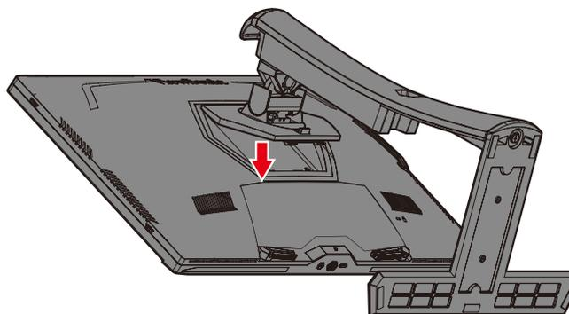
5. Attach the mounting bracket to the VESA mounting holes at the rear of the monitor. Then secure it with four (4) screws (M4 x 10 mm).
